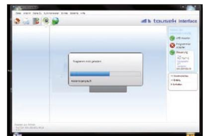
Download the current drive software using the update function and transfer it to the control board.
