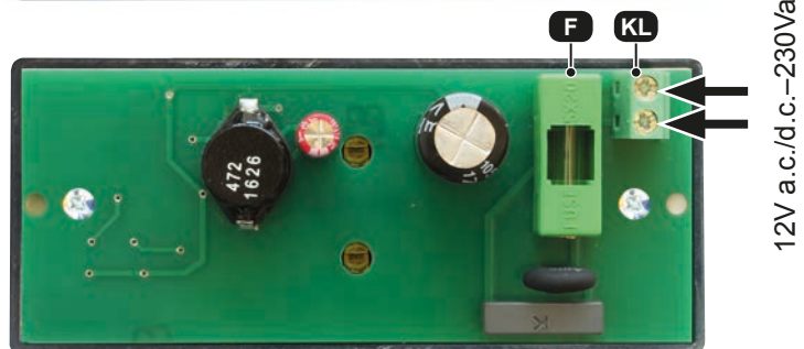
LED blinking lamp 12Va.c./d.c.–230Va.c.
